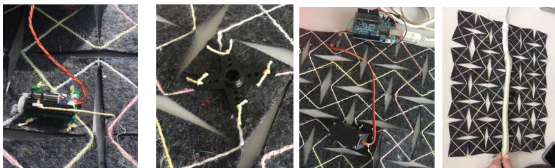
Figure 2 actuation with a DC motor (both left), a linear motor, and a mckibben air muscle.
