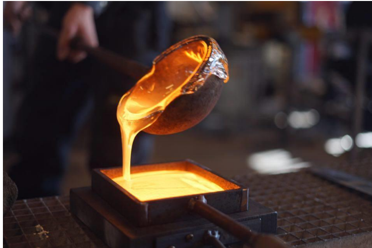
Figure 4 Shaping of glass. Source: Mads Hoby
