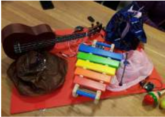
Figure 6: Several Micro:bits used to control servos that are connected to various physical extensions, each designed to make an instrument play.
