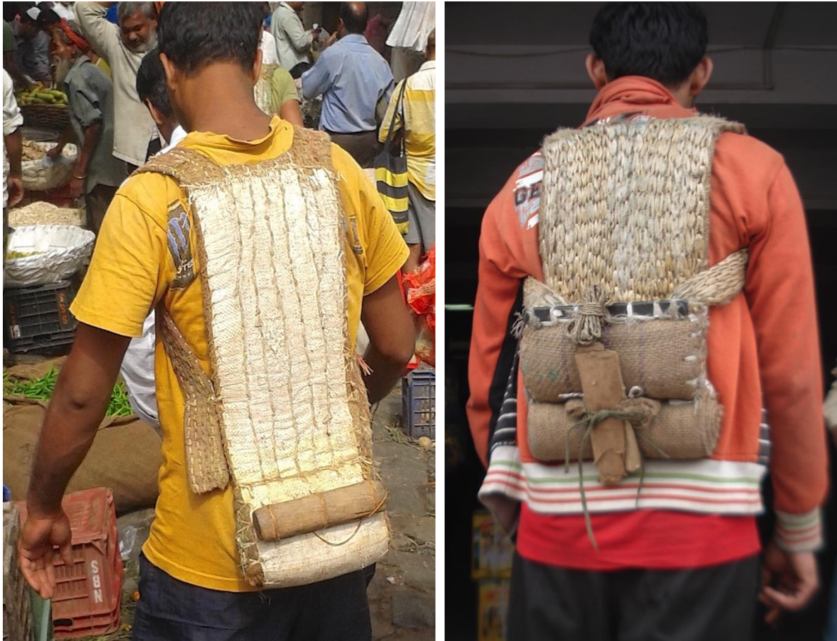
Figure 3 A pitthia and Figure 4 A pitthu; notice the relative height difference between the two object-tool, the position of the support and variation in material, wood in Daryaganj, and rubber belt in Azadpur; also obvious the variation in the joinery of the strap to body of the pitthia and pitthu; Notice the variation in the use of plastic in the two locations. Source: Author
