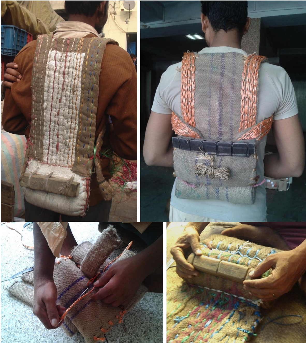
Figure 5 This pitthia has new straps attached in jute atop a plastic sack reinforced body. Figure 6 A month old pitthu, with the user beginning chain-stitch on the straps. Figure 7 Stitching a knot in the middle of the base, which will support the straps. Figure 8 Attaching the wooden support piece. Source: Author
