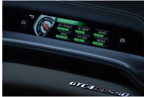
Figure 6 View of the current driving mode through front-seat passenger's infotainment screen in Ferrari GTC4 Lusso. Source: Ferrari (2016)
