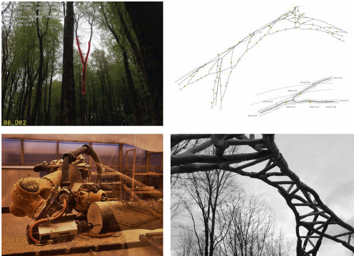
Figure 15-18 The Tree Fork Truss design process of the Woodchip Barn. Natural tree forks are 3D scanned, selected for structural and anisotropic properties, then CNC milled for glue-less on-site joinery. Source: Mollica & Self, 2016.
