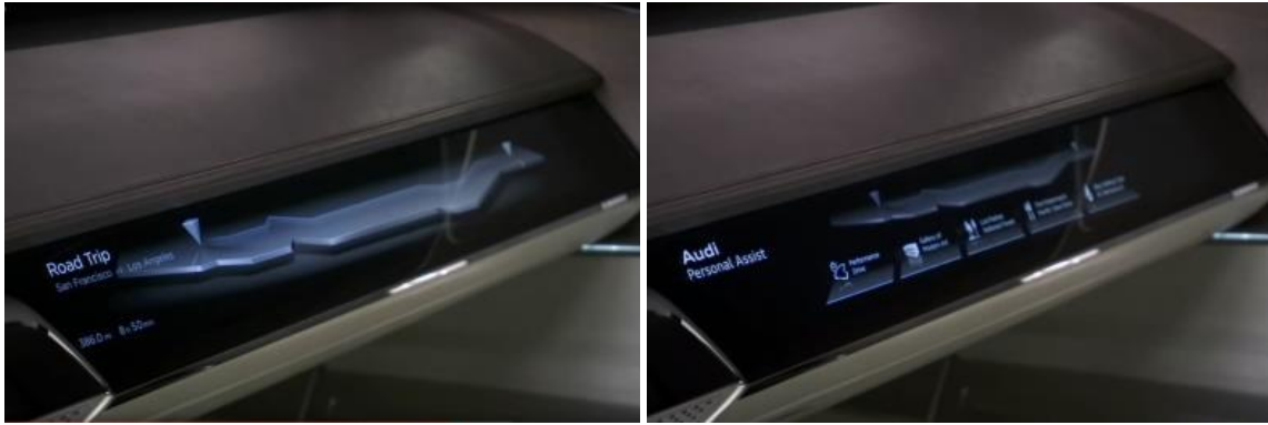
Figure 4 Audi Prologue concept with journey-related information in 'Road Trip' and 'Personal Assist' menus. Source: Carscoops (2014)
