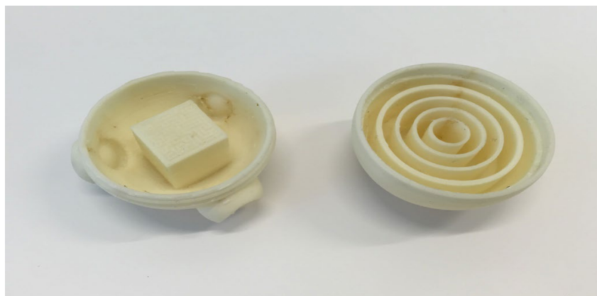
Figure 9. 3D printed sample spheres showing varying wall-thicknesses and intricate details.
