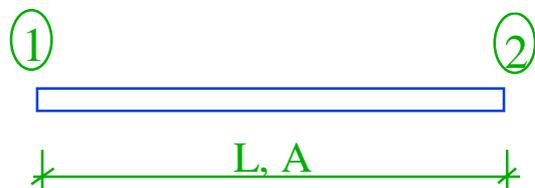
Diagram of a bar element with node 1 fixed ( $u_1 = 0$ ) and node 2 displaced by  $u_2$ . The stiffness coefficients are  $k_{11} = \frac{A E}{L}$  and  $k_{21} = -\frac{A E}{L}$ .
