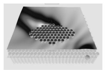
defects and inhomogeneities in the arrangement or diameter of the cylinders.
