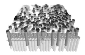
If a disordered array is used instead, we have a Sonic Glass, and with a slow modulation in the lattice parameter we obtain a
