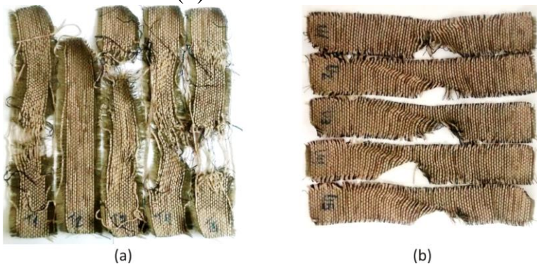
FIGURA 32 – Ruptura trama (a), Ruptura urdume (b) do CHENILLE
