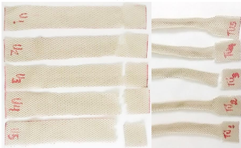
FIGURA 35 – Ruptura vertical (a), Ruptura horizontal (b) do MESH.
