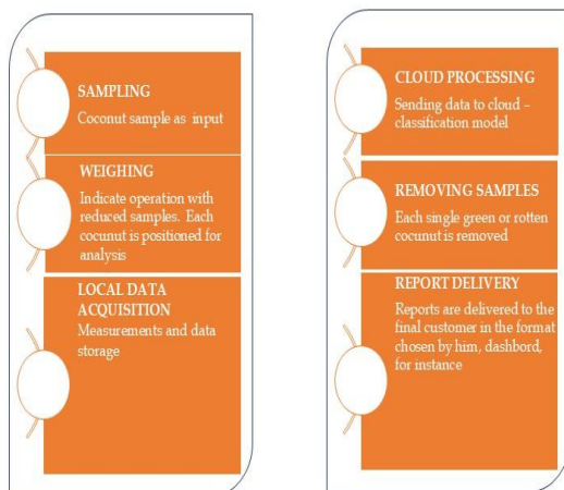
Figura 5: Functional architecture of CAS
