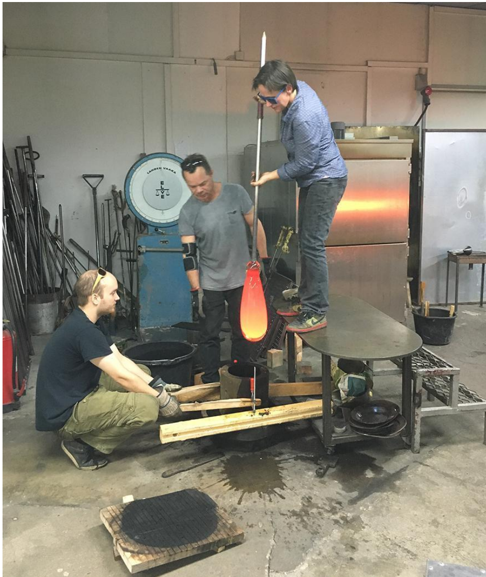
Figure 7 Blowing hot glass into a wooden mould. Photo by the authors.
