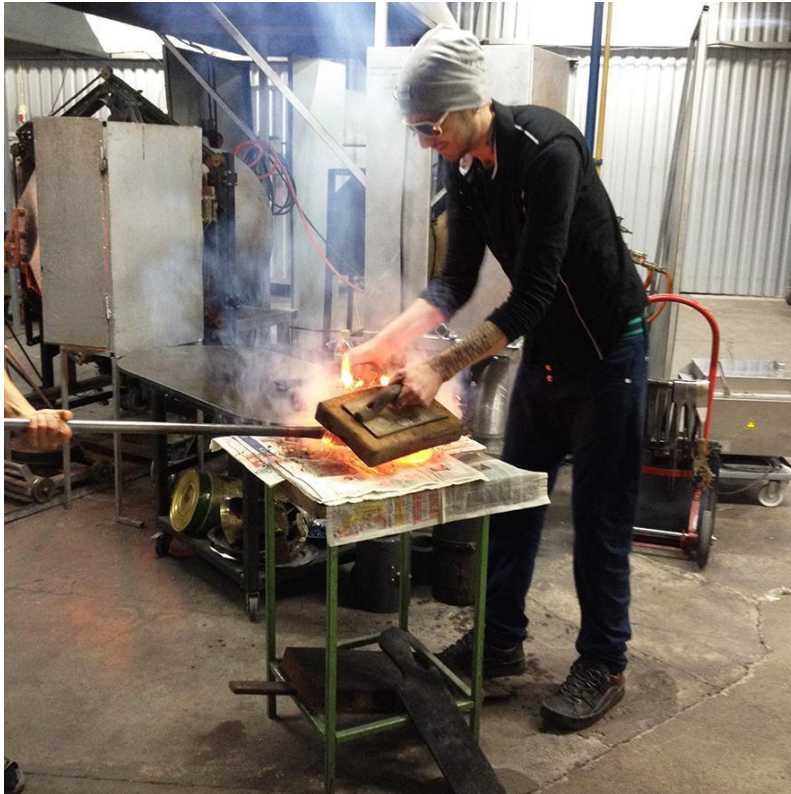
Figure 10 Shaping the blown glass by pressing. Photo by the authors.
