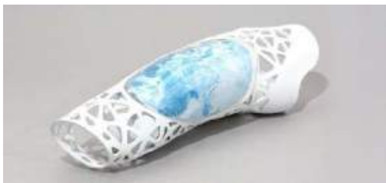
Figure 4: 3D printed prototype – prosthetic limb socket
