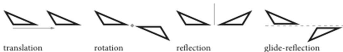
Figure 1 The four symmetry operations in the plane.
